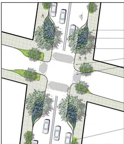
Planted bump-outs will help to manage stormwater running down Ridge
